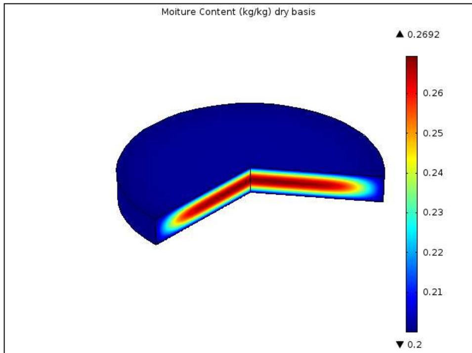
**Figure 6:** Moisture distribution after 60 min of drying
