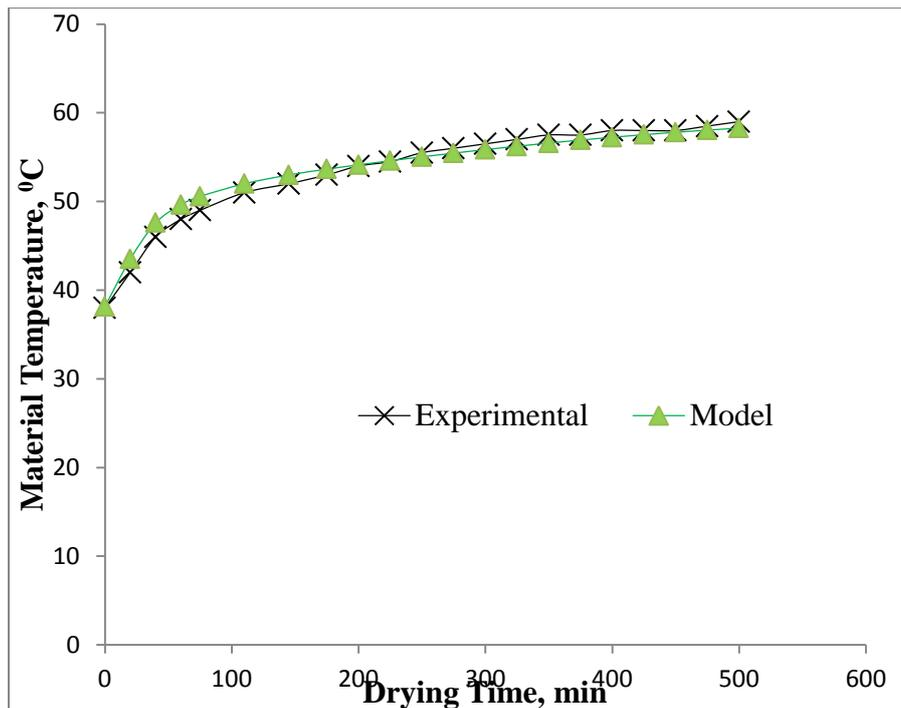
**Figure 2:** Temperature profile obtained for experimental and simulation with shrinkage and temperature dependent diffusivity (for drying air temp,  $T=60^{\circ}\text{C}$  and drying air velocity= $0.5\text{m/s}$ )
