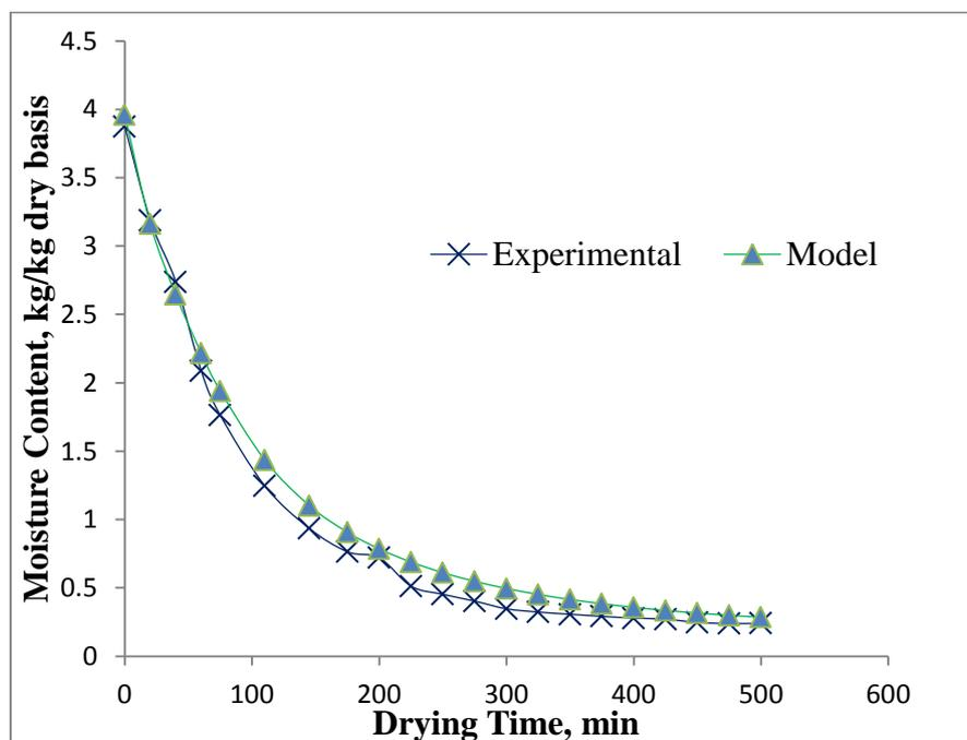
**Figure 3:** Moisture profile obtained for experimental and simulation with shrinkage and temperature dependent diffusivity (for drying air temperature= $60^{\circ}\text{C}$  and drying air velocity,  $V=0.7\text{m/s}$ ).
