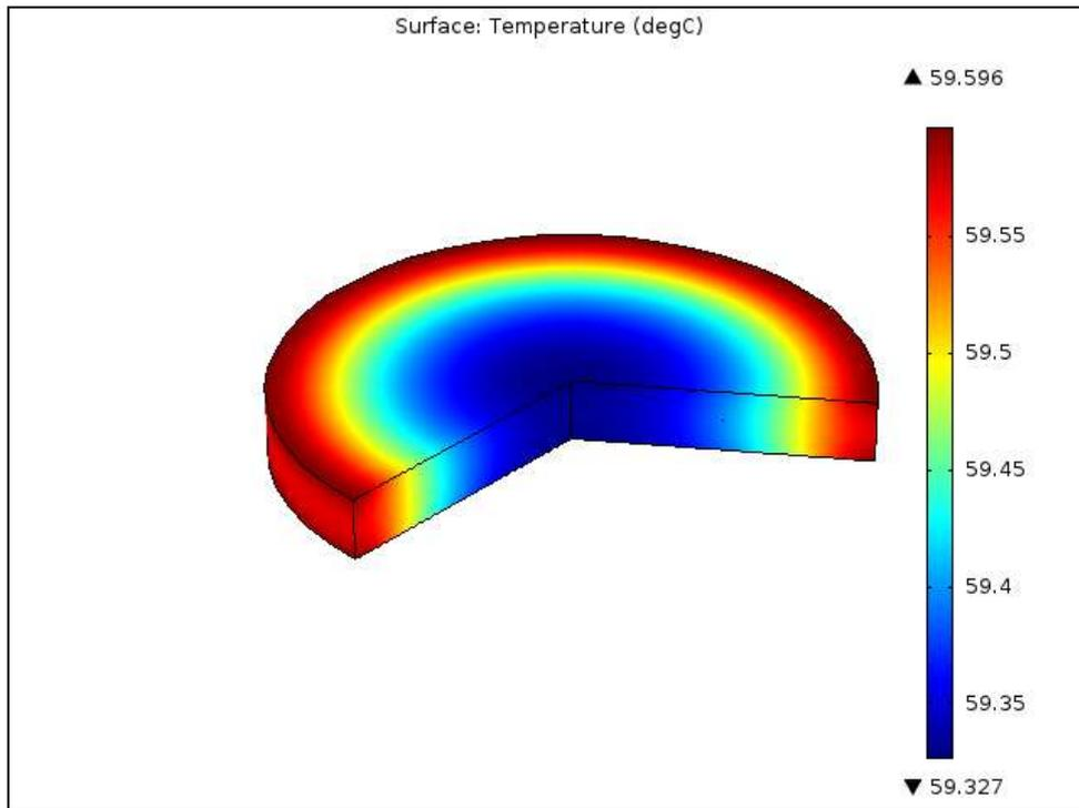
**Figure 5:** Temperature distribution inside the product after 60 mins of drying
