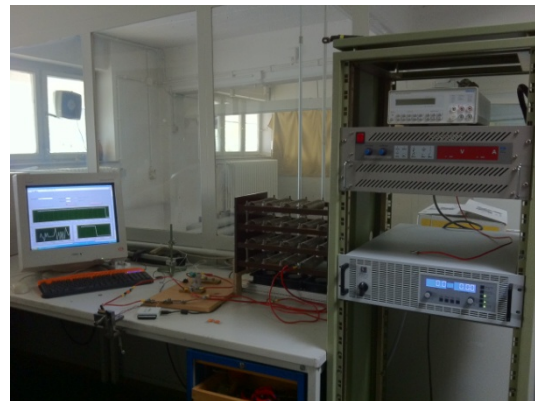
Figure 3. Test setup to take measurements concerning the triggering behaviour of fuses.
