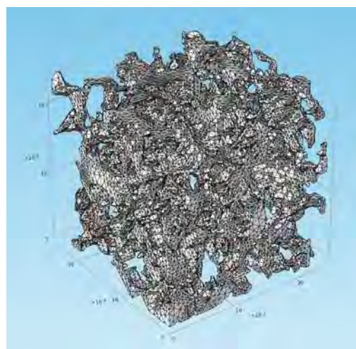
Figure 3. One eighth of original Bentheimer sample: geometry and mesh; L_1=L/2 (cf. figure 2).
