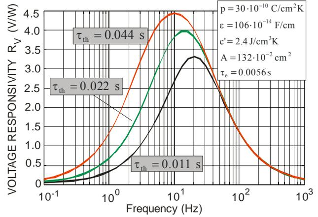
Fig.4. Voltage responsivity of the pyroelectric detector obtained with various thermal time constants  $\tau_{th}$  of the pyroelectric detector. Other parameters of the pyroelectric detector are listed in table 1
