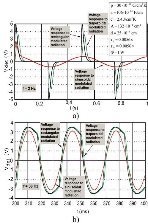
Fig. 6. Voltage response  $V_{det}$  of pyroelectric detector to sinusoidal, rectangular and trapezoidal modulated irradiation of power amplitude  $\Phi = 1$  W and of frequency a)  $f = 2$  Hz, b)  $f = 30$  Hz. Other parameters of the pyroelectric detector are listed in Table 1
