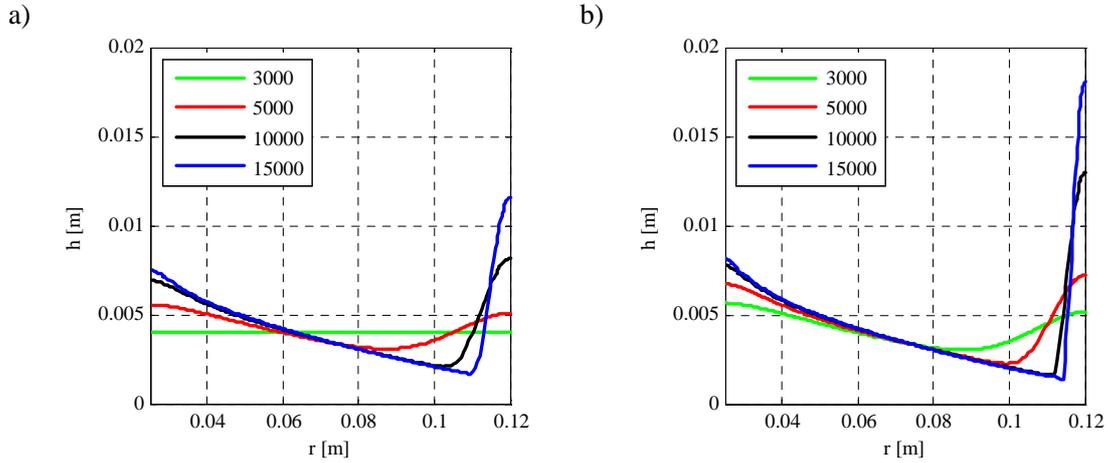
**Figure 1.** Flywheel profiles for a different rotational speeds given in rpms. a) aluminum; b) steel.
