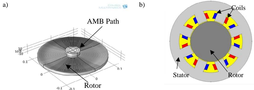
**Figure 5.** Generated geometries: a) complete flywheel rotor; b) AMB
