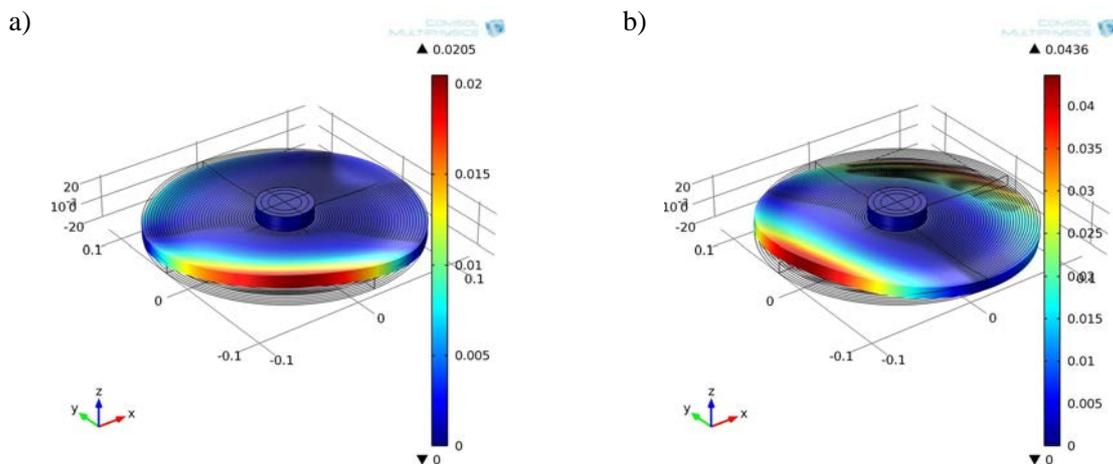
Figure 6. Surface displacement for rotational speeds: a) 3000 rpm; b) 15000 rpm.
