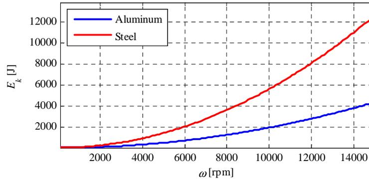
**Figure 3.** Energy stored with respect to the rotational speed for the considered flywheels
