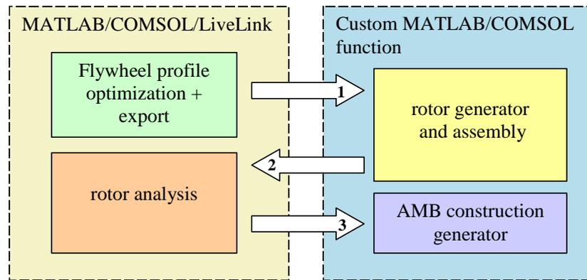
**Figure 4.** Path for automatic generation of flywheel components.
