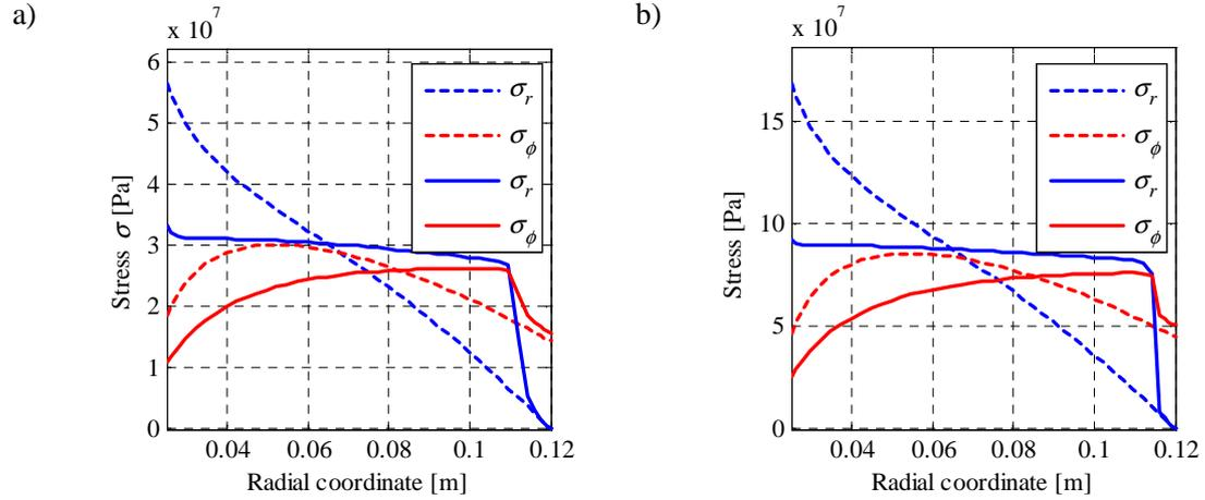
**Figure 2.** Radial (blue) and azimuthal (red) stress components for initial (dashed line) and optimized (solid line) flywheel profiles calculated at 1500 rpm. a) aluminum; b) steel
