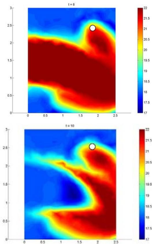
**Figure 6.** Temperature distribution ( $Gr=0$ ;  $Re=1000$ ) in case of supplying hot (top) and cold (bottom) air. The circle marks the location of the ‘sensor’ used as input for the Relay i.e. switch.
