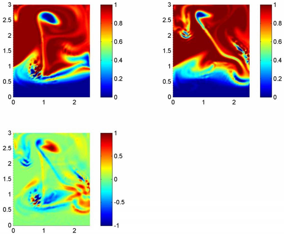
Appendix C: Scaled temperature distribution after 60 time steps (case:  $Gr = 2.5 \cdot 10^7$  and  $Re = 1000$ ); Top Left: Air supply temperature equals 1 (22 °C); Top Right: Air supply temperature equals 0.975 (21.9 °C); Bottom: Air temperature difference between the top figures where 0 means no difference; +1 means 4 °C hotter; -1 means 4 °C colder
