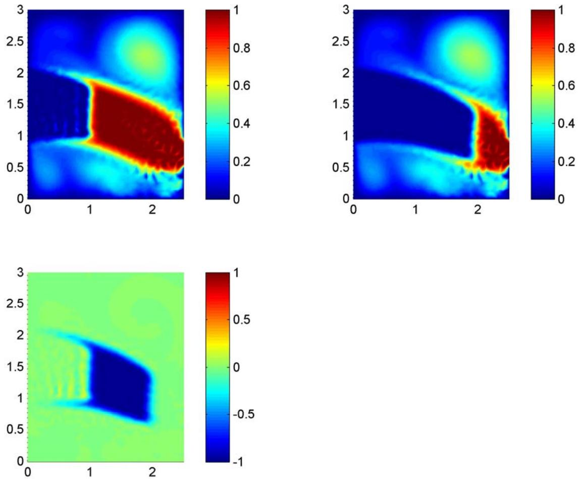
Appendix D: Scaled temperature distribution after 30 time steps with on/off controller case  $Gr = 0$  and  $Re = 1000$ ; Top Left: The 'sensor' temperature thresholds are respectively below 0.30 and above 0.50. Top Right: The 'sensor' temperature thresholds are respectively below 0.32 and above 0.48. Bottom: Air temperature difference between the top figures where 0 means no difference; +1 means 4 °C hotter; -1 means 4 °C colder
