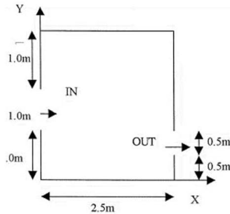
**Figure 1.** The geometry of the airflow problem.
