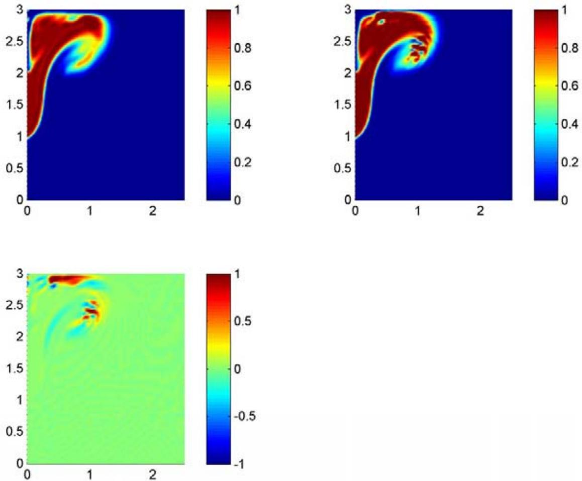
Appendix A: Scaled temperature distribution after 10 time steps (case:  $Gr = 2.5 \cdot 10^7$  and  $Re = 1000$ ); Top Left: Air supply temperature equals 1 (22 °C); Top Right: Air supply temperature equals 0.975 (21.9 °C); Bottom: Air temperature difference between the top figures where 0 means no difference; +1 means 4 °C hotter; -1 means 4 °C colder
