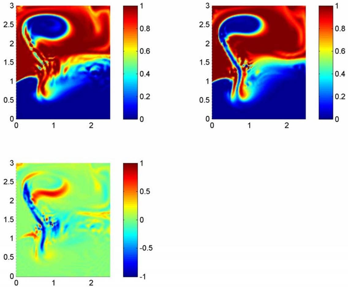
Appendix B: Scaled temperature distribution after 40 time steps (case:  $Gr = 2.5 \cdot 10^7$  and  $Re = 1000$ ); Top Left: Air supply temperature equals 1 (22 °C); Top Right: Air supply temperature equals 0.975 (21.9 °C); Bottom: Air temperature difference between the top figures where 0 means no difference; +1 means 4 °C hotter; -1 means 4 °C colder
