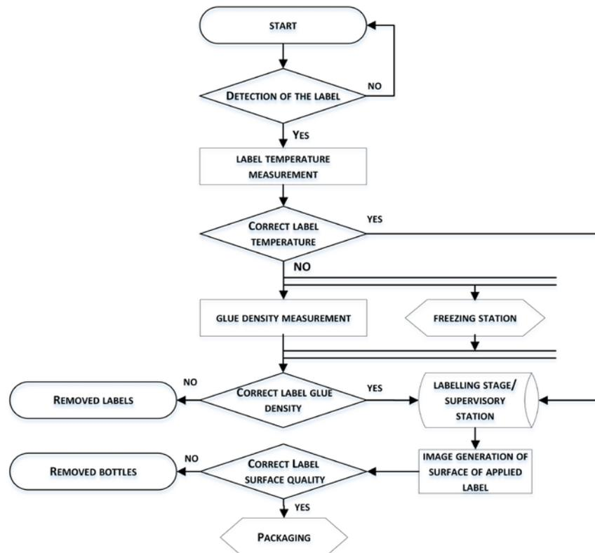
Fig. 3. Scheme of label defects detection
