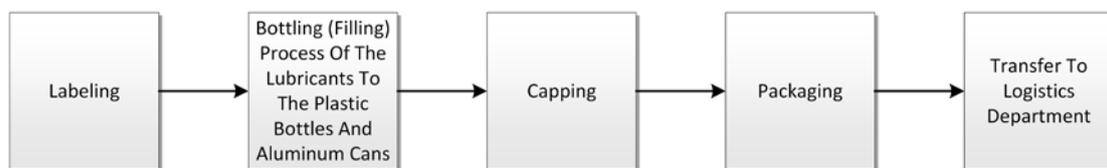
Fig. 1. Workflow of the filling process
