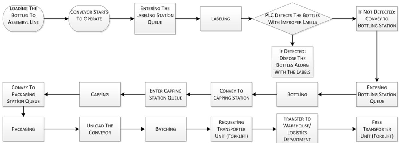
Fig. 2. Detailed process flow at filling facility
