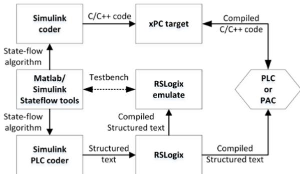
Fig. 4. Workflow of the model-based design [10]
