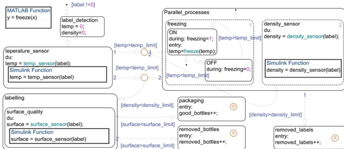
Fig. 5. Chart of the process algorithm
