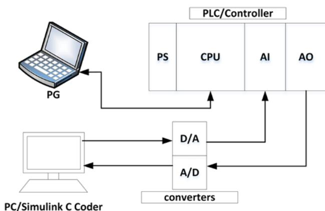
Fig. 6. Connection between the PLC and PC/Simulink C coder during HIL simulation
