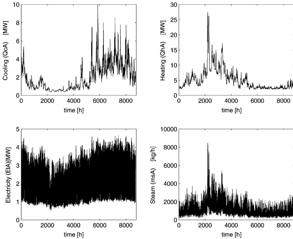
Fig. 6. The non-controllable inputs of the model: cooling, heating, electricity and steam needed for the Academic Hospital against time.
