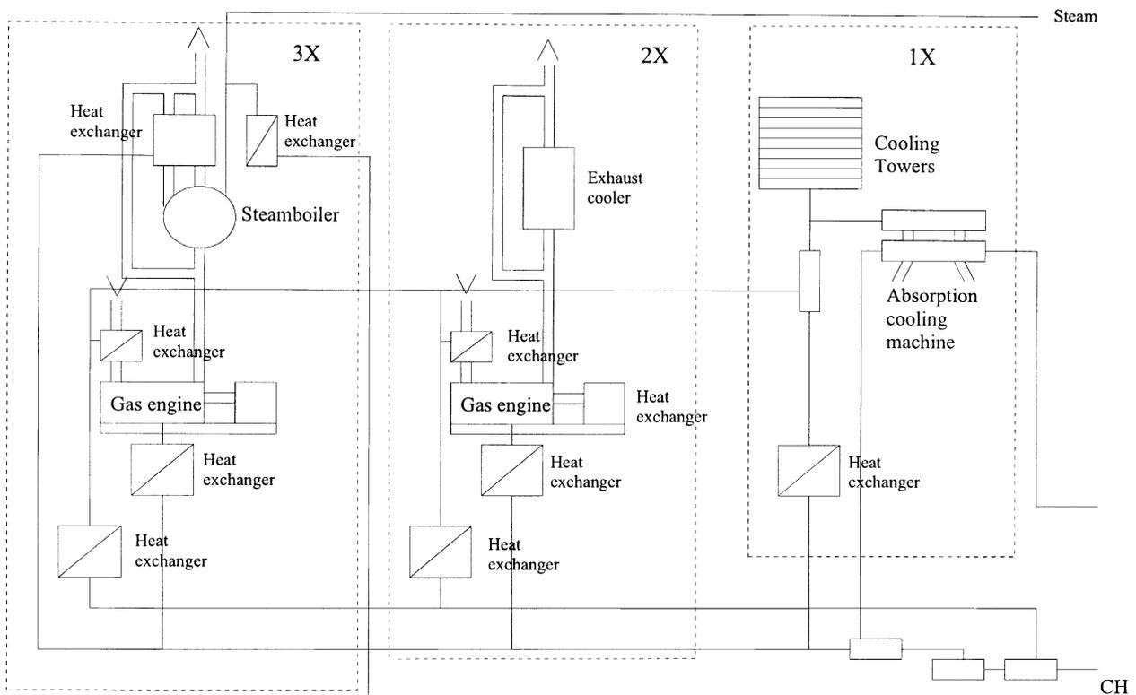
Fig. 2. The power plant (the seven cooling units, connected with the absorption chiller are not shown in this figure).
