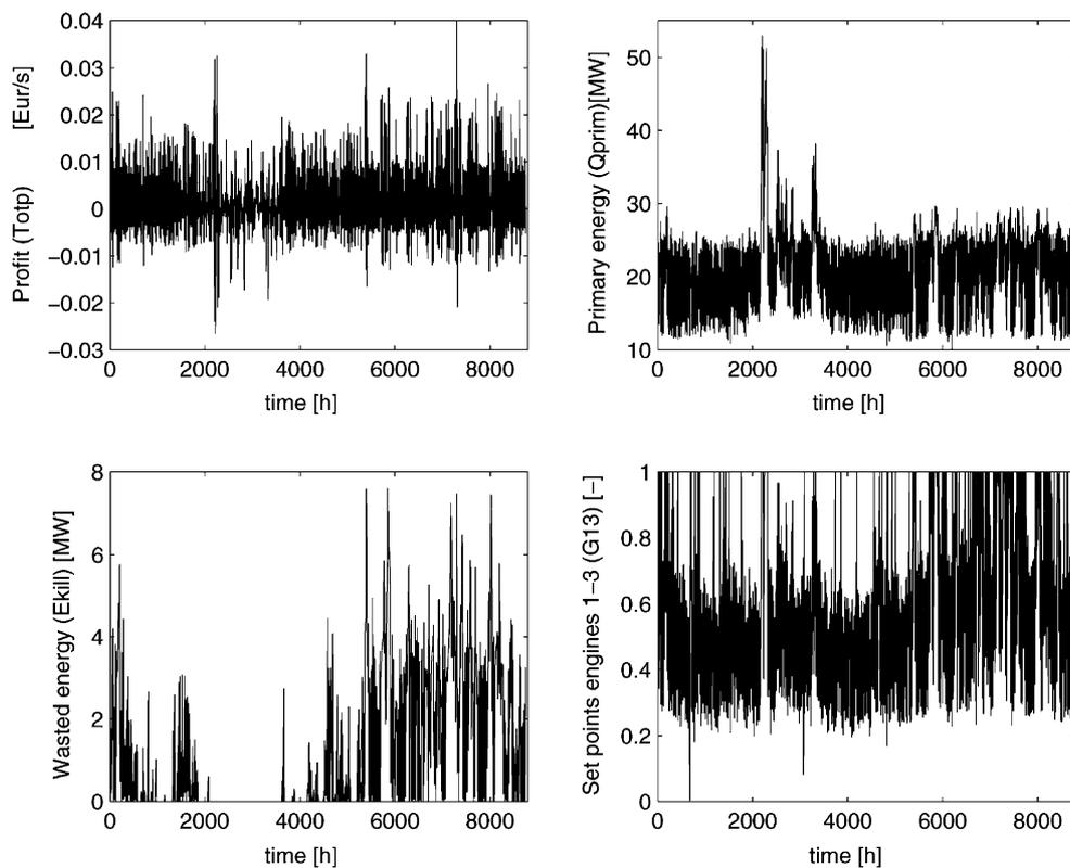
Fig. 7. The output signals: profit, used primary energy, wasted energy and set point of gas motors 1–3 against time.
