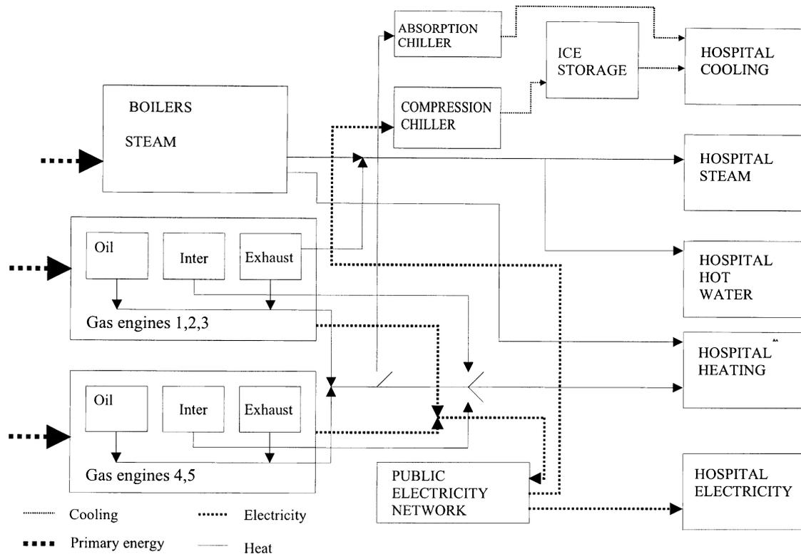
Fig. 3. The energy flows of the power plant and cooling installations.
