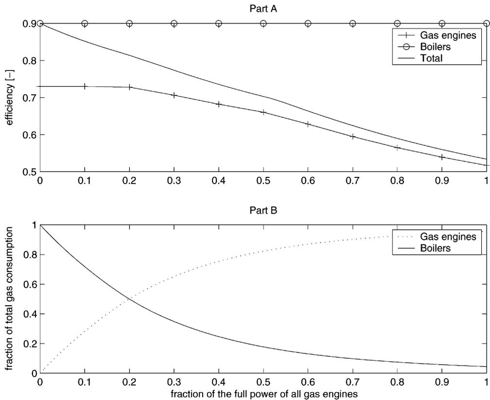
Fig. 9. (A) The efficiency of the boilers and gas motors; (B) the fraction of gas consumption of the boilers and gas motors.
