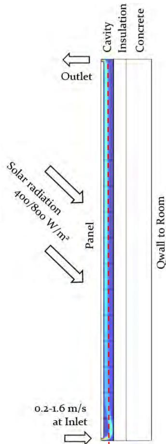
**Figure 3:** Schematization of the heat balance model
