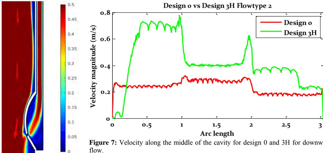
**Figure 7:** Velocity along the middle of the cavity for design 0 and 3H for downward flow.
