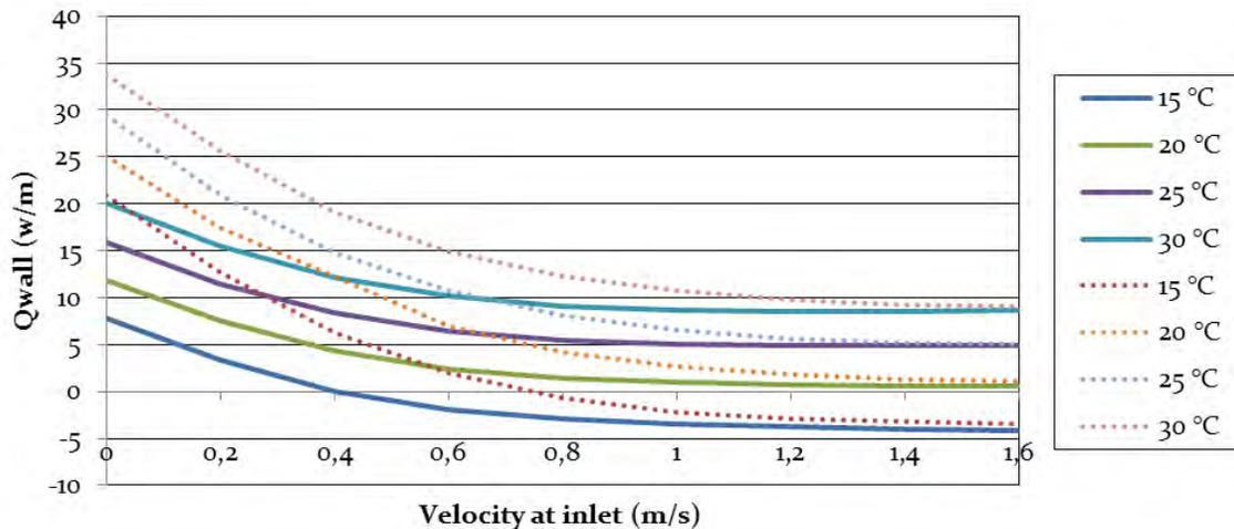
**Figure 4:** Graph of the heat transfer at the inside of the internal wall to the room, set off to the velocity at the inlet (dotted lines are 800 W/m<sup>2</sup>).
