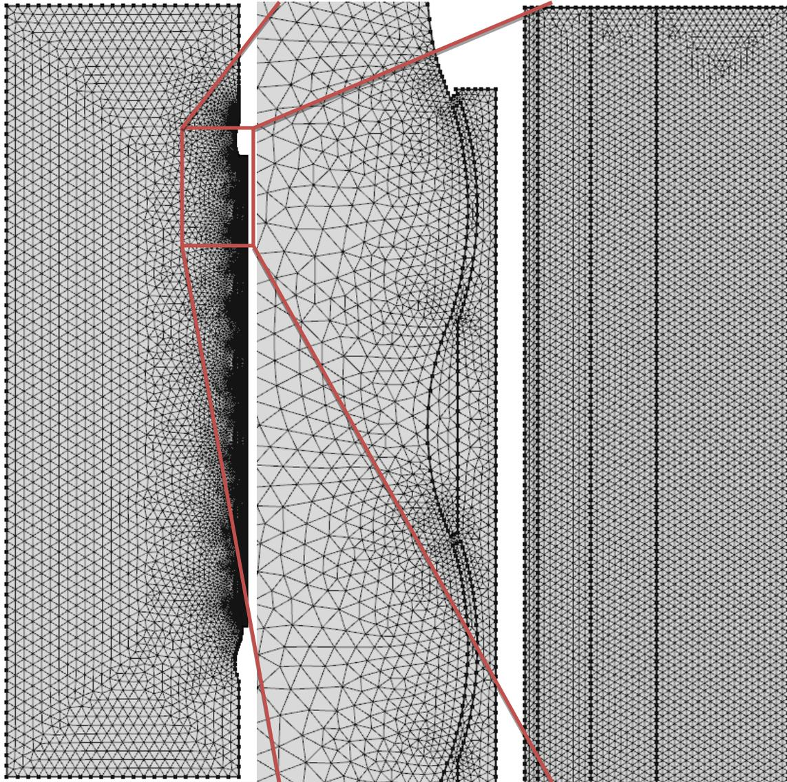
**Figure 14:** Mesh of design 4A with curved facade elements.
